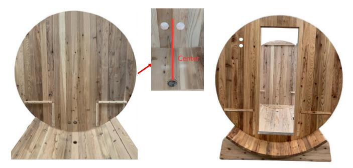
7. Place additional 9pcs staves on each side of the barrel. Use 36pcs 3\*30mm screws to fix the 18pcs staves to the front & back panel.
