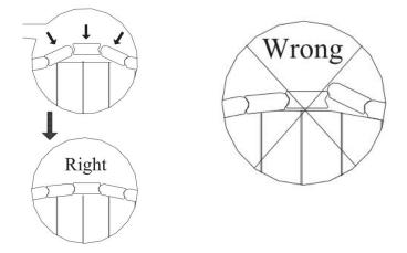
After the top piece is correctly installed, fix the remaining staves with 4\*40mm screws.
