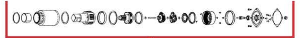
Exploded view of RAD gearbox
