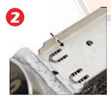
Place shroud over radiator and mark on upper/lower metal lips where the bolt holes sit. Drill into metal lips at marked locations.
