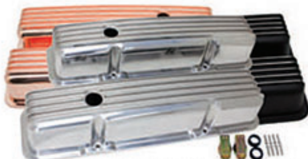
CHEVY SMALL BLOCK - RETRO FINNED W/HOLE 1958-86, 283-305-327-350-400 BAFFLED HZ-6720-3-POL Polished HZ-6031-3-POL Polished HZ-6720-3-PBK Black HZ-6031-3-PBK Black HZ-6720-3-C Chrome HZ-6031-3-C Chrome HZ-6720-3-COP Copper HZ-6031-3-COP Copper TALL H: 3-11/16" SHORT H: 2-9/16"
