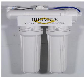
This is the main unit, comprising two filter housings, membrane housing and control devices. The unit should be installed against a vertical surface, in a position which allows for the filters and membrane to be replaced periodically. The module should be as close as possible to the storage tank (10) and faucet (14), to give a good flow of water. Using the bracket as a template, mark the position of the fixing screws, leaving at least 40mm of free space below the housings for filter changes.
