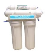
This is the main unit, comprising two filter housings, membrane housing and control devices. The unit should be installed against a vertical surface, in a position which allows for the filters and membrane to be replaced periodically. The module should be as close as possible to the storage tank (10) and faucet (14), to give a good flow of water. Using the bracket as a template, mark the position of the fixing screws, leaving at least 40mm of free space below the housings for filter changes.
