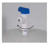
Simply wind four wraps of P.T.F.E. around the threads of the reservoir inlet / outlet. Offer the vacant threaded port of the valve onto the threads and tighten clockwise. **Do not over tighten** – this is not a high pressure joint.
