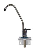
Select a position for the tap on the counter or sink shoulder. The faucet should be located in a position that gives a flow of water into the sink bowl. Ensure (check) that you have enough room below the desired position to connect the tubing (11) to the tap. Using a centre pop (or nail) mark where the centre of the tap stud will be and drill a 12mm hole through the surface. Secure the tap in place by using the fixing kit provided.
