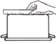
Check pans for flat bottoms by using a straight edge
