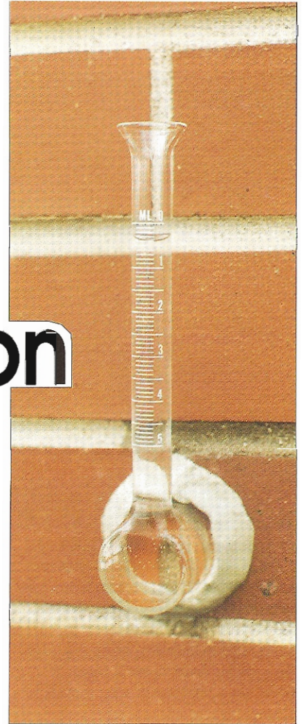
RILEM or MAT tubes are pipelike devices. The tube or stem portion is graduated from 0.0 to 5.0 ml. The volume of water absorbed over a specified time is read from this graduation.
