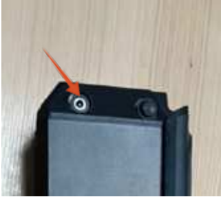
Battery Charging Port
