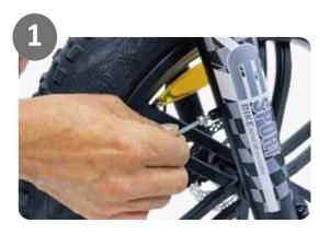
1.Remove the screws on both sides of the front fork arms.
