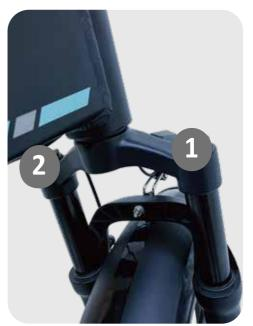
The preload adjustment knob(2), located on the top of the left side of the suspension fork. To soften the ride, subtract resistance by turning the preload adjustment knob counterclockwise, in the direction of the small "-" on the knob. To make the suspension suffer when going over bumps, add resistance by turning the preload adjustment knob clockwise, in the direction of the small "+" on the knob.
