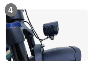
4. Wrap the clamp around the fork without touching the brake rotor, insert the bolt and tighten. Repeat on the other side.
