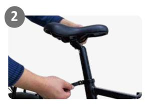
2.Insert the seat post into the seat tube.
