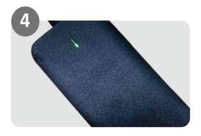
4.Once fully charged, the charging indicator light turning green. Unplug the charger from the wall outlet first and then remove the charger output plug from the battery charging port.
