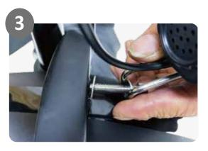
3. Pass the bolt through the headlight mount, fender mounting point and the fork arch mounting point, then tighten the nut.
