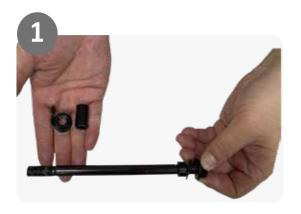
1. Locate the axle skewer and unscrew the nut and long cylinder.
