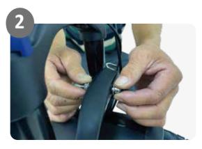
2.Remove the headlight mounting hardware from the fork arch.
