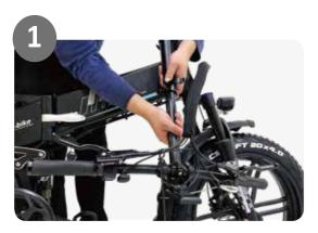
1.Insert the handlebar into the stem.
