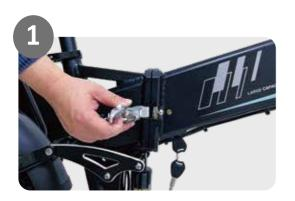
1. Open the quick-release lever on the frame.
