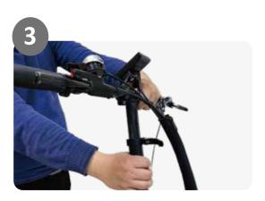
3. Adjust the height of the handlebar.
