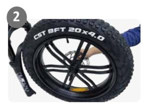
2. Pass the skewer through the axle from the brake disc side and make sure the brake disc is on the left of the bike.
