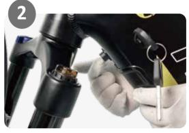
2. Press the release button and hold the battery.
