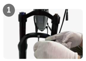
1.Remove the headlight mounting hardware from the fork arch.
