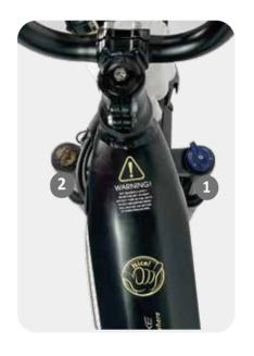
The preload adjustment knob(2), located on the top of the left side of the suspension fork. To soften the ride, subtract resistance by turning the preload adjustment knob counterclockwise, in the direction of the small "-" on the knob. To make the suspension suffer when going over bumps, add resistance by turning the preload adjustment knob clockwise, in the direction of the small "+" on the knob.
