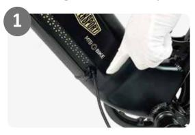
1.Remove the rubber cover on the charging port and charge the battery directly.
