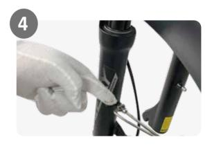
4.Remove the screws on both sides of the front fork arms and then tighten the iron bar.
