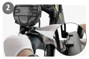
2.Pass the bolt through the headlight mount, fender mounting point and the fork arch mounting point, then tighten the nut.
