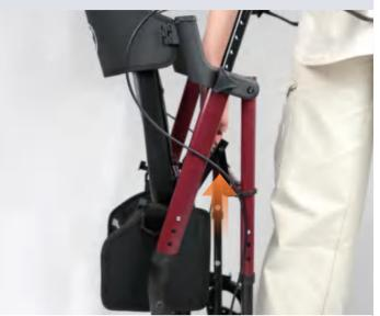
Pull up the black metal brace inside the basket to fold the rollator.
