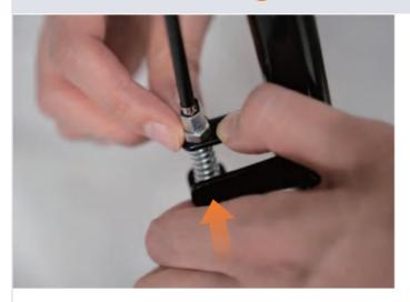
Use one hand to press the iron piece under the spring upward.
