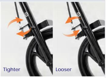
Turn the nut clockwise to increase braking force; Turn the nut counter-clockwise to decrease braking force.
