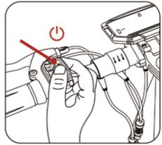
Using an NFC key card: Put the NFC key card against the NFC sensing area on the right back of the display.
