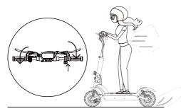
4.Release the accelerator and the kinetic energy recovery system (KERS) initiates automatically to brake slowly; And squeeze the brake lever for a sudden brake
