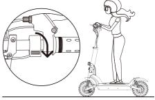
3.When the scooter starts to move forward, put both feet on the deck and press the accelerator. (The accelerator initiates once the speed exceeds 3 mph.)
