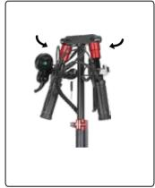
Step 2: Release the quick release clamp on the front tube. Press down the handlebar to the bottom.
