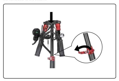
Step 3: Pull out the folding lever and pull the folding clamp to fold down the front tube.
