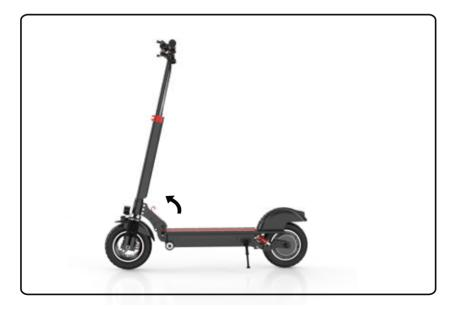
Step 3: Expand the handlebar upward and keep it straight.
