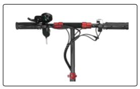
Step 4: Adjust the handlebar to the suitable height and then tighten the quick release clamp.
