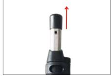
Remove the plastic covers on the front axles and stem.
