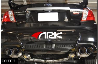
10. It is recommended that someone hold the someone else tightens down all of the nuts and bolts to the proper torque specs (Figure 7)
