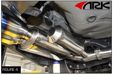
5. Spray the rubber insulator and metal hanger on the driver side muffler with a lubricant (Figure 4)
