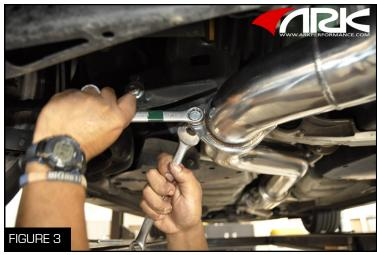
4. Bolt the resonator pipe to the Y-Pipe with the supplied gasket, nuts, and bolts using both 16 and 17 mm socket wrenches (Figure 3)
