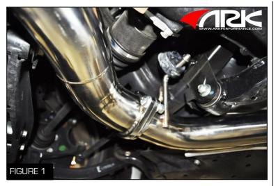
1. Spray the rubber insulator and metal hanger on the resonator pipe with a lubricant (Figure 1)
