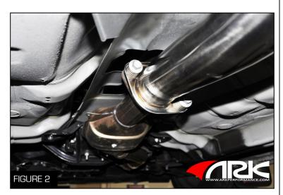
3. Bolt the resonator pipe to the OEM catalytic converter pipe (or test pipe) with the OEM donut gasket, nuts, and spring loaded bolts using both 12 and 14 mm socket wrenches (Figure 2)
