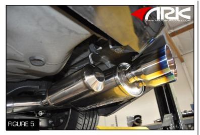
7. Spray the rubber insulator and metal hanger on the passenger side muffler with a lubricant tips and mufflers in the proper position while (Figure 5)
