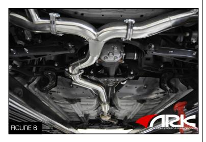
9. Bolt the two mufflers to the Y-Pipe with the supplied gaskets, nuts, and bolts using both 16 and 17 mm socket wrenches (Figure 6)
