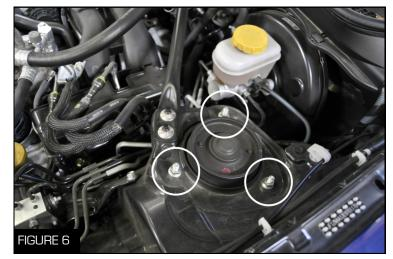
7. Unbolt the top of the strut using the 12 mm socket wrench and slowly lower the strut out of the car (Figure 6)
