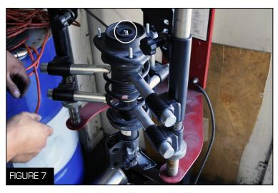
6. The brake assembly will tilt outwards once 8. Hold the spring with the spring compressor and unbolt the center nut with a 17 mm socket (Figure 7)
