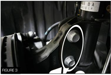
1. Properly jack up the vehicle on flat, level 4. Unbolt the strut from the brake assembly (Figure 3)
