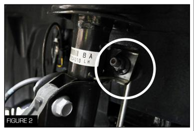
3. Unbolt the sway bar end link using the 17 mm wrench (5 mm hex key may be necessary to stop stud from spinning) (Figure 2)
