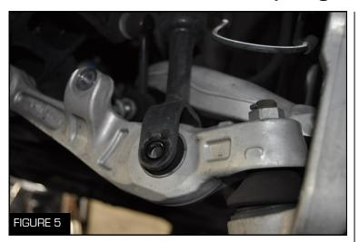
arm using a 17 mm socket wrench for both the using a 17 mm socket wrench (Figure 7) nut and bolt (Figure 5)
