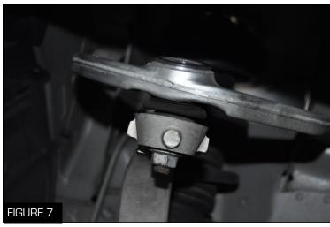
7. Unbolt the strut tower from the suspension 9. Unbolt the nut on the top suspension part
