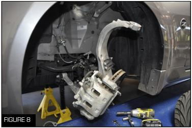
10. Push the brake assembly down and out and pull the OEM spring out (Figure 8)
