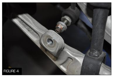
6. Unbolt the sway bar end link using a 17 mm socket wrench (Figure 4)
