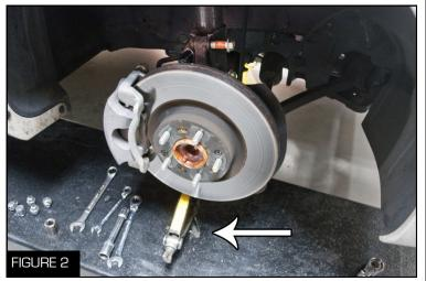
3. Place the OEM scissor jack under the brake rotor to support it before unbolting anything (Figure 2)
