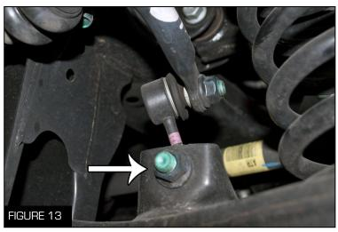
1. Remove the rear wheels using the proper 3. Unbolt the sway bar using a 17 mm socket socket or key for the lug nuts or wheel locks wrench and move the link out of the way (Figure 13)
