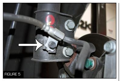
6. Unbolt the brake line using a 12 mm socket wrench and move it out of the way (Figure 5)
