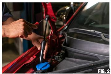
2. Using the small hook tool, remove the hood struts from the hood hinges.
