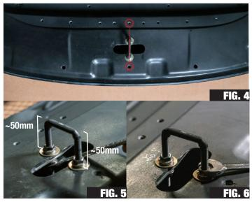
2. The adjustable hood latch catch will need to be adjusted to fit your vehicle. Use the 12mm wrench to adjust the nuts. We recommend that you adjust the height to approximately 50mm from the base to the top. Make sure to keep the height level on both ends. The latch catch should also be following the line created by the two holes indicated in Fig. 4.
