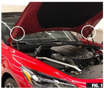
1. Have an additional two people hold up the hood as you remove the bolts from the hinges holding the hood. After taking off the hood, take off the two rubber stoppers from the front portion of the hood.
