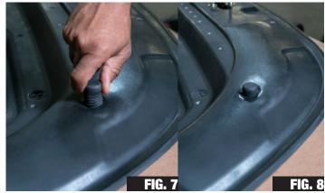
3. Take the OEM / Stock rubber stoppers and fit them in the appropriate holes. Turn the stoppers all the way into the holes until the threads are no longer visible. You may need to adjust the height of the stoppers later for better fitment.
