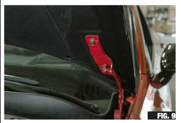
4. Lift the hood hinges, and place the R-Spec Hood on top while lining up the hood's bolt holes with the hinges' bolt holes. Using the bolts (from step 1), screw in the bolts to hold the hood in place but do not fully tighten bolts yet.
