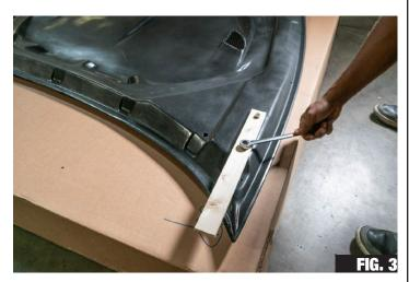
1. Remove all plastic packaging material from the hood. You should see that there is a wooden block on each corner. Remove the bolts and save them for the installation. Do not use the OEM / stock bolts for the R-Spec hood.
