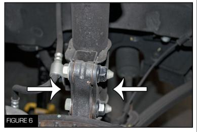
7. Spray the two nuts and bolts with a lubricant to make them easier to unbolt (Figure 6)
