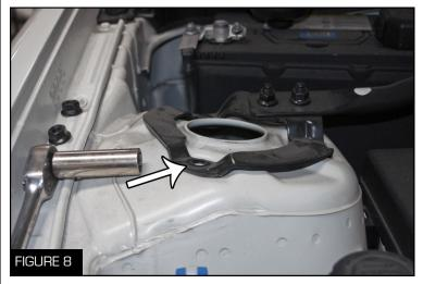
10. Unbolt the three bolts on the strut using a 14 mm socket wrench and remove the strut/spring from the car (Figure 8)
