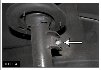
5. Unbolt the sway bar end link from the strut using a 19 mm socket wrench (Figure 4)
