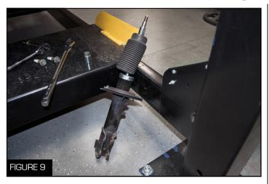
11. With the strut off of the vehicle, remove the top piece and take the OEM spring off (Figure 9)
