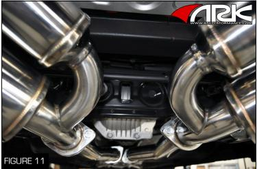
17. Bolt the driver side muffler to the rear pipe with the supplied nuts, bolts, and flange gaskets using both 16 and 17 mm socket wrenches, then do the same for the passenger side (Figure 11)
