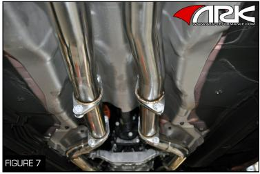
10. Attach the X-Pipe to the OEM catalytic converter pipes with the OEM nuts and flange gaskets using a 17 mm socket (Figure 7).
