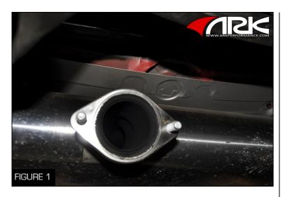
1. Unbolt the muffler from the resonator pipe using a 17 mm Socket Wrench (Figure 1)
