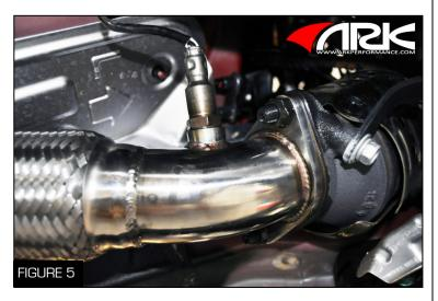
8. Optional parts: Bolt the down pipe (specific to the driver or passenger side) to the OEM primary catalytic converter with the OEM nuts, bolts, and flange gaskets using a 17 mm socket wrench per side (Figure 5)
