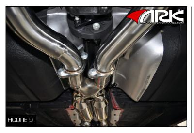
14. Bolt the passenger side rear pipe to the X-Pipe with the supplied bolts, nuts, and flange gaskets using both 16 and 17 mm socket wrenches (Figure 9)
