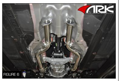
9. Optional parts: Bolt the test pipes to the down pipes with the provided nuts, bolts, and flange gaskets using both 16 and 17 mm socket wrenches (Figure 6)
