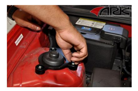
6. Put the Strut Brace Bar base on with the (2) holes next to each other facing the rear of the vehicle. Loosely fasten them with the factory nuts on both passenger and driver side.
