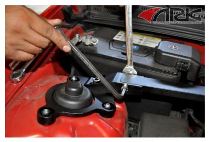
10. Loosely fasten the long hex key bolt with an 8mm hex key and a 15mm wrench.
