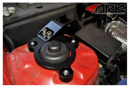
7. Mount the top mount adapter to the base with the (2) supplied hex key bolts on both passenger and driver side.
