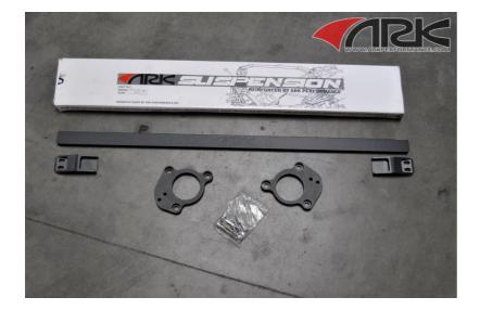
1. Inspect the contents of the box to make sure that there are no damages and that the bar, (2) top mount adapters, and (2) bases, and the bag of hardware are included (2 long hex key bolts, 2 short hex key bolts, and 2 serrated nuts).
