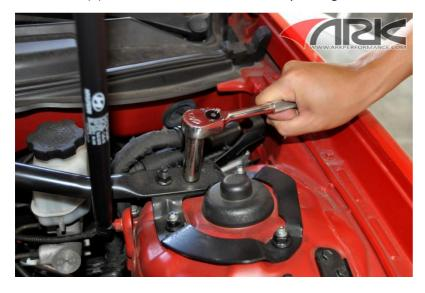
4. Unbolt the (2) OEM nuts on the strut brace bar on the driver's side to make removing the brace easier.
