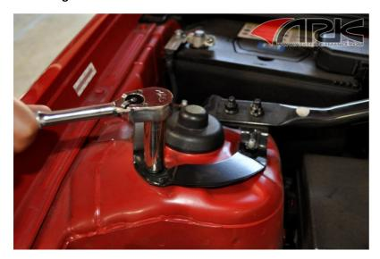
2. Remove the (3) OEM nuts on the OEM strut brace bar with a 14 mm socket on the passenger's side. These nuts will be used later with the Strut Brace Bar from ARK Performance.
