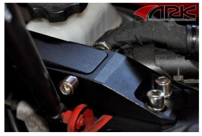
9. Place the bar into the opening on both adapters. Slide the long hex key bolt though the adapter and through the bar, fasten it with the supplied serrated nut on the side facing the rear of the vehicle.
