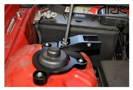
8. Loosely tighten the hex key bolts with an 8mm hex key on both sides.
