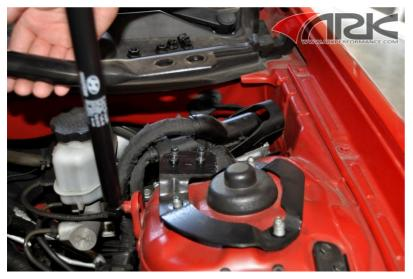
5. After the (5) OEM nuts are removed from the driver's side. Lift up the bar from the driver side and then remove the passenger side bar and base. Then remove driver side base.
