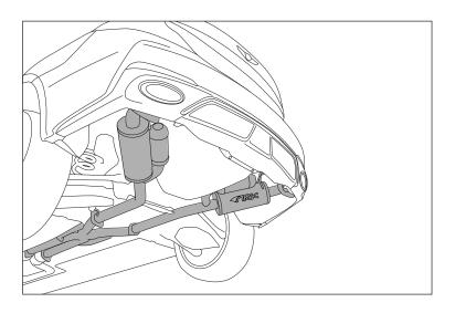
2. Install the ARK Performance GRiP System onto your vehicle. Please install with the appropriate gaskets. The tips should extend well into the exterior exhaust tips built into your vehicle's diffuser.
