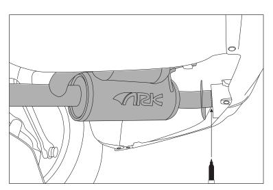
3. Using a felt tip pen or marker, mark the GRiP System's piping at the edge of the inner exhaust tip. Take the mufflers off of the vehicle.
