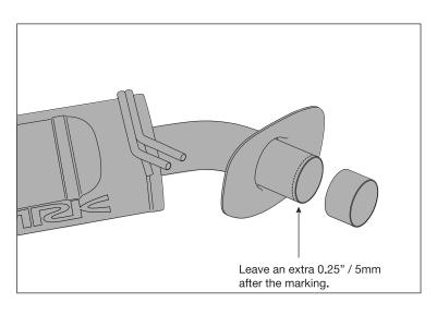
4. For the ideal cut, please cut a quarter inch or 5mm into the diffuser. This will allow the exhaust gas to expel safely past the diffuser.
