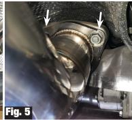
1. Lubricate the rubber insulator towards the front of the vehicle and the hanger on the front pipe (Fig. 4). Replace the gasket with the included triangle gasket. Bolt the three nuts of the front pipe to the triangle flange (Fig. 5). Insert the front pipe hanger into the rubber insulator.
