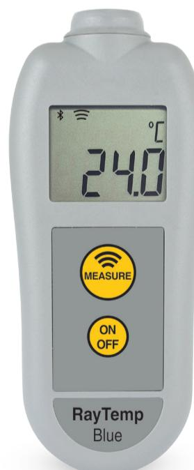
**INSTRUMENT OPERATION** - Simply switch the instrument on and the display will show 'rdy'. Aim the RayTemp Blue at the target and press the 'MEASURE' button to measure the surface temperature. When the button is released the reading is automatically held and 'HOLD' will be displayed.
