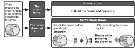
\* By locking the crown by screw, a screw down crown can prevent malfunction and increase water resistance. \* Be careful not to screw the crown in by force as it may damage the slots of the crown.
