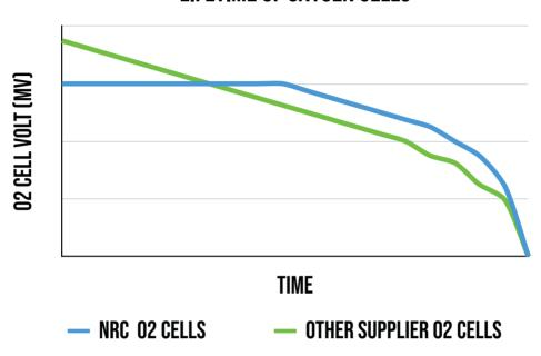
While the initial output voltage of NRC galvanic oxygen sensors (blue) may appear slightly lower compared to certain counterparts from other manufacturers (green), it exceeds the specified target value for a longer time. Furthermore, this variance in output has no impact on the overall service life, which remains unaffected by the lower starting point of the voltage curve.
