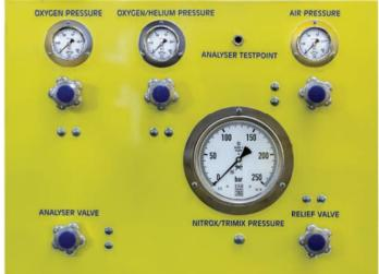
If high oxygen concentrations are required, quick and flexible gas mixtures are essential, or Trimix is a significant part of your daily gas logistics, we have the perfect solution for you. The extremely flexible Blending Panel can be customized and configured to meet all your needs. Choose the required inputs and outputs, and we'll configure it for you. All in the familiar NRC quality and safety. Explore the possibilities and find your personalized Blending Panel.
