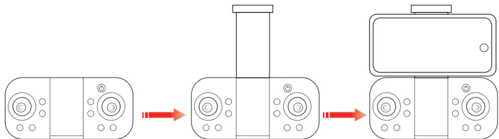
The ALLY's controller has a built in controller holder. To unfold this, pull up from the bottom of your controller. You can slide the top of the controller holder to adjust for phone size.
