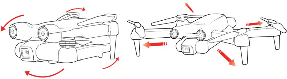
To unfold your ALLY, pull the folding arms away from the body. The arms rotate out, and will make a 'clicking' noise when deployed. Push the arms back in to turn ALLY into a portable drone! Do not force the arms, and be gentle when moving them.
