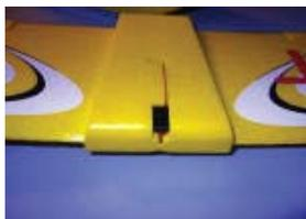
Next, locate the servo connector on the wing. Gently pull it out.
