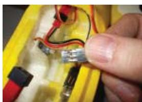
Slide the connector onto the pins, with the silver side down.
