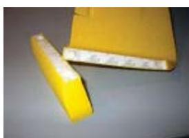
Next, install the wing tip. Find the small tip, and remove the 3M tape backing from the wing.
