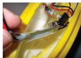
Gently pull the ESC out to make connecting easier.
