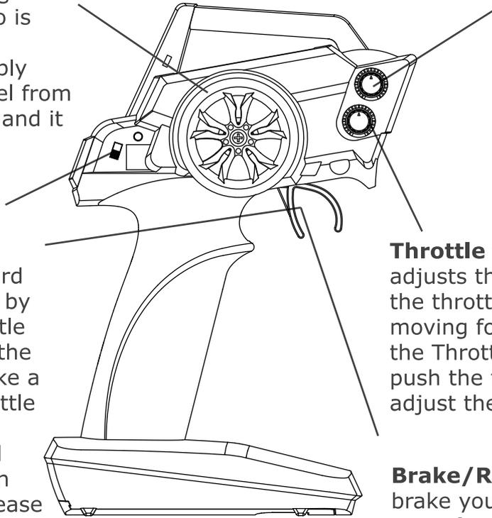
**Throttle trim:** The throttle trim adjusts the neutral (centre) point of the throttle control. If your model is moving forward or backwards when the Throttle Trigger is at neutral, push the trim button and this will adjust the neutral point.
