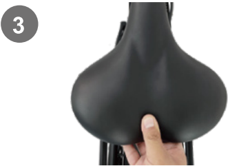
3. Adjust the seat and the head of the seat is parallel with the top tube.
