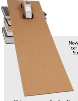
Now comes the fun part. Get your timing device ready and put your car at the top of the ramp. When you let the car go, start the timer. Stop the timer when the back of the car goes off the ramp.
