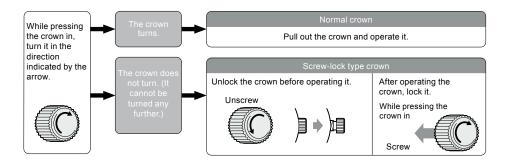
\*If your watch has a screw-lock type crown, the crown screws into the watch to prevent malfunction and increase water resistance. \*Be careful not to screw the crown in by force as it may damage the slots of the crown.
