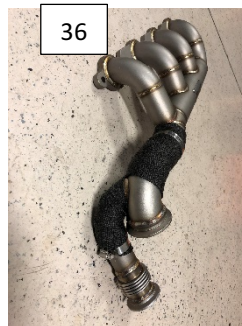
36 Test fit exhaust manifolds using 9/16" ratchet wrench. We recommend wrapping the area shown on the PS with the supplied wrap. Reinstall steering column and starter (leave starter wiring off for future step). Note DS clearance of WG tube to body as well as PS log to cradle. Depending on wear of engine mounts, you may want to add some clearance in these 2 areas with a small dimple above the DS WG tube and small grind on PS Cradle under the Log. This may not be necessary but can be done for additional clearance to prevent vibration.
