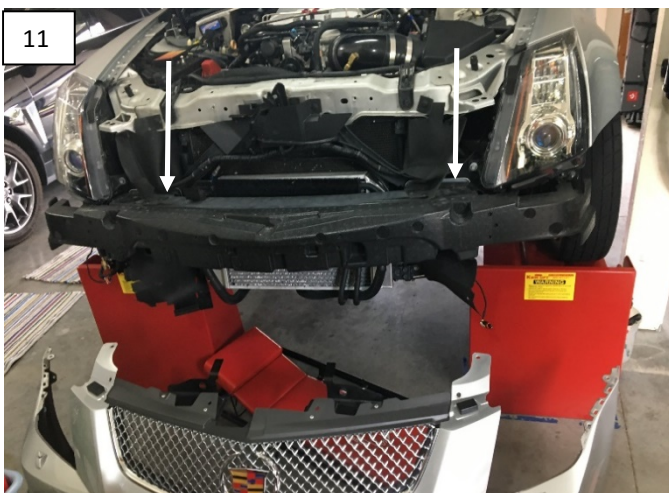
11 Remove eight bolts in front impact bar, use 13mm socket on 7 and 13mm ratchet wrench on upper left bolt, right side. Remove impact bar.
