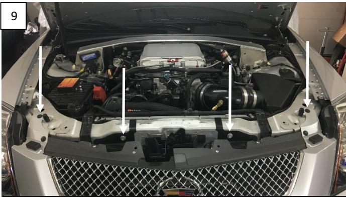
9 Unplug right and left fog light. Remove 2 retainer clips and 2 bolts with 10mm socket and ratchet in front bumper cover and lift bumper cover off.
