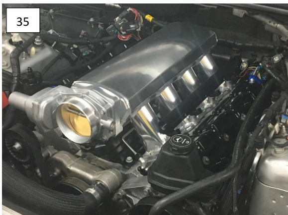
35 Remove blue tape and install new intake with injectors/fuel rails and throttle body. Torque tb to 89in/lbs and intake to 44in/lbs first pass and 89in/lbs final pass. Connect fuel line to fuel rail.
