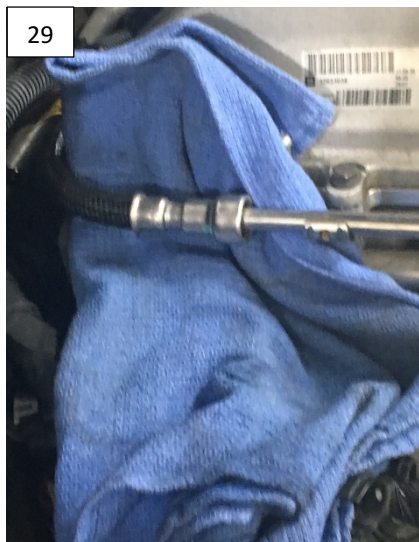
29 Disconnect fuel line using quick disconnect tool.
