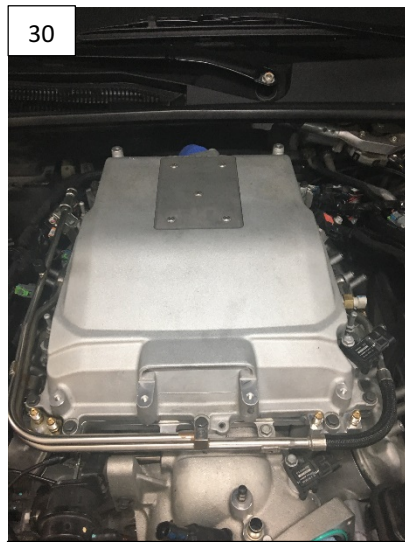
30 Remove coolant lines to supercharger intercooler brick on back of supercharger and disconnect 8 plugs/hoses from supercharges and lid.
