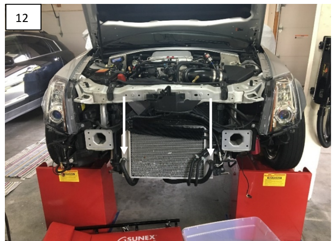
12 Drain intercooler by removing one of the hose clamps and pulling off hose. Use bucket to catch coolant. When coolant is drained remove other hose and drain.
