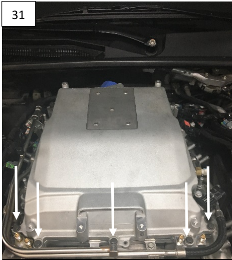
31 Remove 17 supercharger lid bolts using 10mm socket and extension. Lift lid off (coolant may drain from the rear intercooler brick lines).
