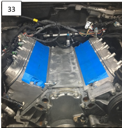
33 Tape off intake ports on heads with blue painters tape to keep out foreign objects.
