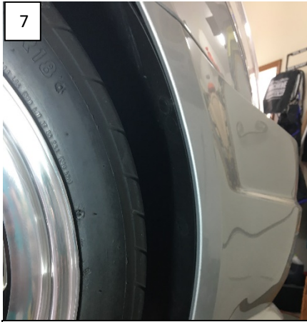
7 Remove 8 retainer clips in each fender well and remove fender well liner.
