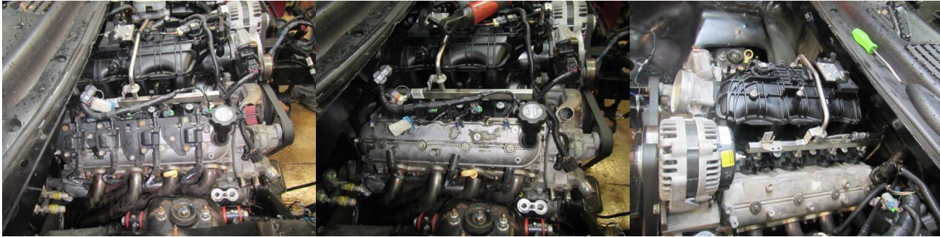
Step 9: Remove coil brackets, spark plugs, spark plug wires and oil dipstick
