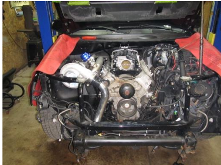
Step 18: Clock turbo and install hot-side intake pipe, oil drain facing down
