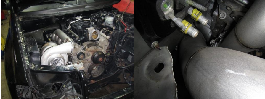
Step 16: Bolt on turbo and down pipe
