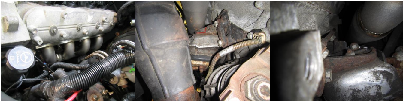
Step 12: Drivers side header (note, check exhaust clearance)
