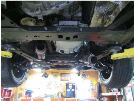
Step 6: Remove existing exhaust system
