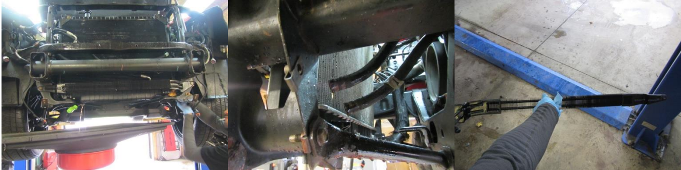
Step 5: Remove front power steering cooler
