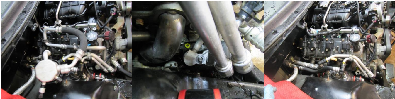
Step 7: Have the AC system properly evacuated. Once done properly, Remove ac condenser and lines and evaporator and coolant tank
