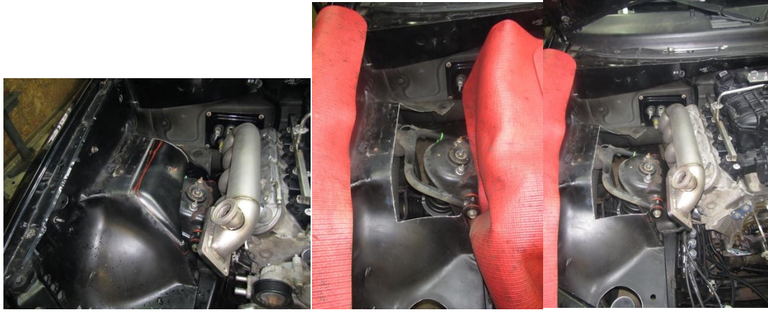
Step 15: Cut inner fender for hot side and turbo clearance
