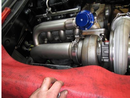
Step 17: Install waste-gate and clamp turbo to down pipe
