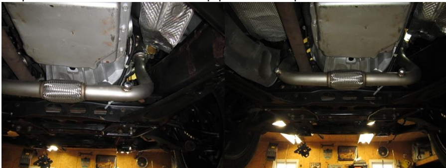
Step 14: Assemble the crossover pipe and clamps
