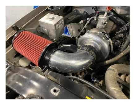
9.) Install the fabricated coolant overflow tank over on the passenger side fender in the OEM slot. You will use a self tapping screw to secure the other bracket.
