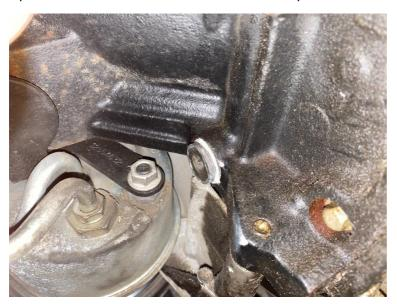
4.) Install the exhaust crossover pipe to each manifold using the supplied 2.5" V-band Clamps and copper v-band gaskets at each connection. This can be broken into the 2 pieces for ease of install. The slip connection is a double joint slip fit that will allow movement while containing the exhaust.
