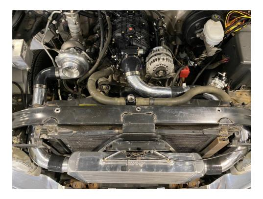
8.) You will attach the 4" 90\* intake tube to the compressor inlet of the turbo and the supplied air filter at the other end using the supplied 4" straight coupler. The short leg of the 4" tube goes into the Turbo connection.
