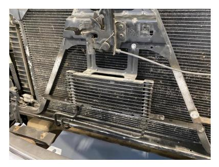
3.) Remove the (1) lower 10mm bolt holding the bottom portion of the power steering cooler, and move the bottom of the bracket just inside the hood latch brace as shown below for extra clearance to the intercooler.
