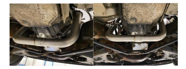
5.) With the manifolds and the crossover installed, tighten down both v-band clamps ensuring both flanges are properly aligned with the copper gaskets in place and fully seated. Next tighten down the exhaust manifolds after the crossover connections are snug. Tighten the exhaust manifold bolts down from the center first, working your way out. Torque to 18 ft/lb.
