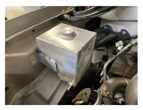
10.) Next is to install the new Coolant fill location. This must be in this location as it has to be the highest point in the system. Mark as we shown below leaving yourself enough hose to fit up to the neck of the Fill T.
