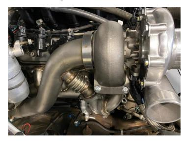
12.) Back under the car we will install the second piece of the downpipe now after the first section is attached to the turbocharger and the wastegate. Earlier model trucks will use the 2-bolt flanged pipe and later model trucks the pipe with the ball flange. Shown below is the earlier model on a 2005 truck.
