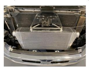
5.A) We supply 2 additional brackets as shown below to mount to the bottom of the intercooler. These brackets are optional with their main goal to give you a location to mount a larger Tru-Cool 40k Transmission cooler which we highly recommend to help keep your transmission temperatures down. Please refer to the photos below for orientation of these brackets, mounting location off the bottom of the intercooler and how the optional Tru-Cool trans cooler can mount!
