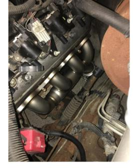
2.) Install the Passenger side exhaust manifold from the turbo kit re-using the factory gaskets or new OEM gaskets with the m8x1.25 30mm long bolts supplied in the turbo kit or OEM bolts if you desire. Leave loosen enough to wiggle the manifold, do not secure it down tightly at this
