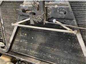
5.) Install the Intercooler to the bracket via (2) m8x1.25x30mm bolts as shown below.
