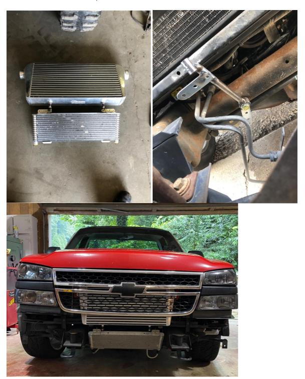
6.) Trim the plastic shown below around the headlight area so our cold-side tubes can pass around the radiator to the intercooler.
