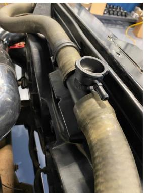
11.) Run the supplied  $\frac{1}{4}$ " Hose from the outlet on the Fill Tee to the Overflow tank, securing with the spring clamps as shown
