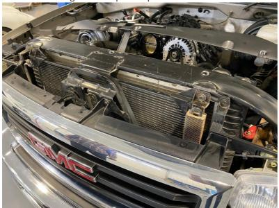
2.) Remove the factory transmission cooler from the mounting location via the top (2) 10mm bolts and the (2) lower push clips. Push down and out of the way for now if you are keeping this cooler. If replacing with a larger Tru Cool style, you can remove the transmission cooler at this time. Remove the lower brace for the transmission cooler via the (2) 10mm bolts.
