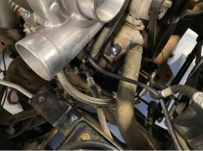
11.) Going back now secure the wastegate inlet clamp we left loose earlier allowing the wastegate to rotate for assembly.
