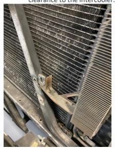
4.) Bolt the intercooler bracket to the (2) open holes on the hood latch bracket using (2) m8x1.25x30mm bolts and (2) M8 nuts on the back side.
