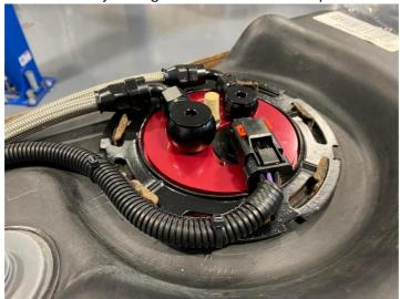
4.) Cleanly route the Feed hose, Return Hose, and Electrical harness out from the tank area.
