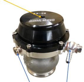
Top Port. Leave vented open unless using a boost controller.
