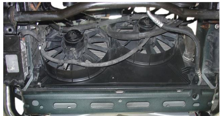
Re Install Fans
