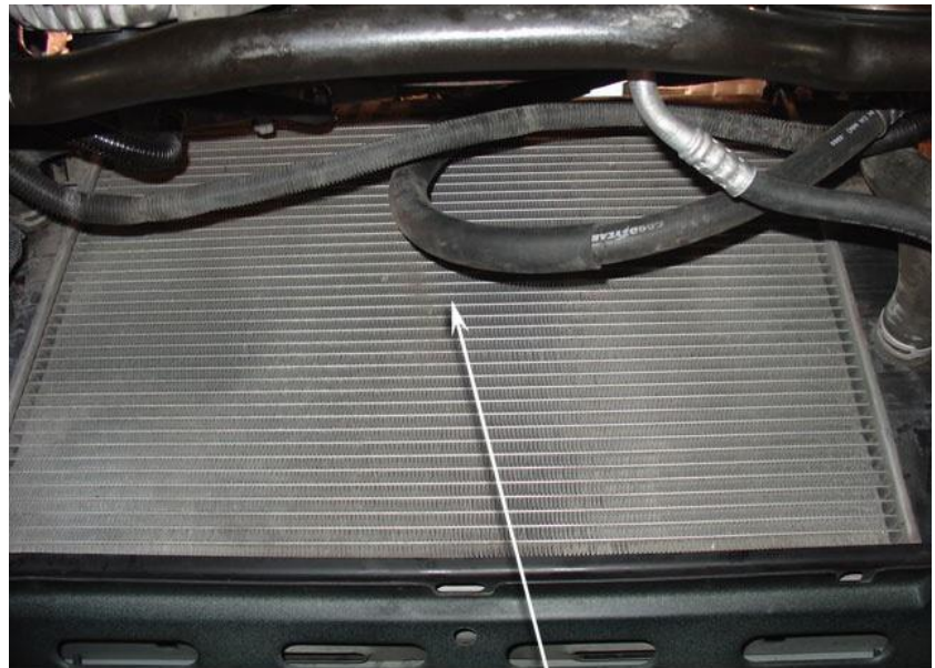
Radiator Cooling Fans Removed
