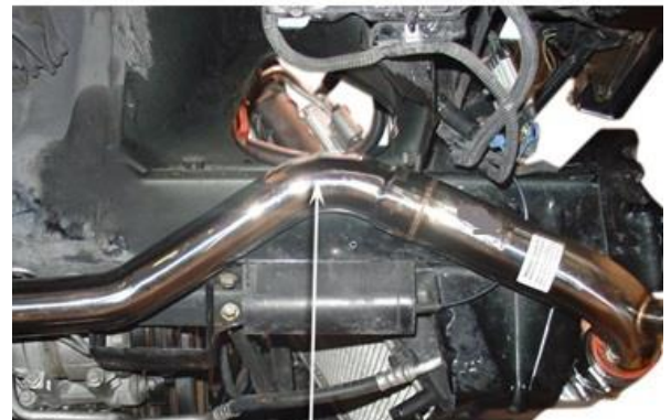
RHS Discharge Duct
