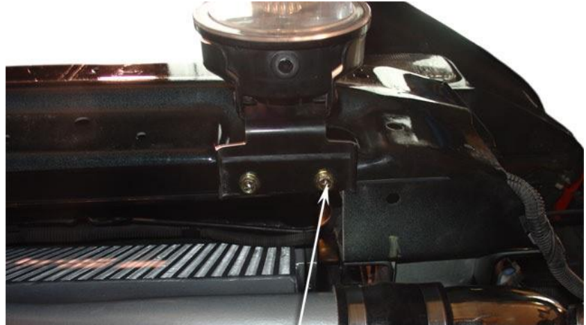
Install 2nd 6mm x 1.0 x 20mm Bolt, 6mm x 1.0 Washer & Nyloc nut
