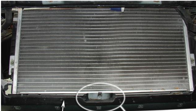
Lower Radiator Support Panel This Area
