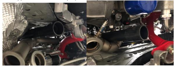
**Step 13:** Prepare Turbochargers for Installation. Please view the following photos below for the proper clocking orientation. You will clock your turbocharger housings from their out of the box orientation by loosing the (6) bolts on the inside edge of the exhaust housing and the 8 bolts on the inside edge of the compressor housing. Once these are loose you will be able to spin both housings to get in your desired positions.
