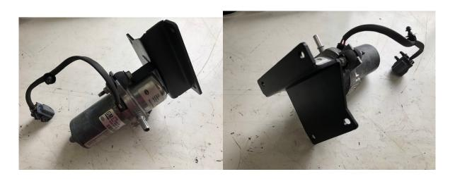
**Step 40:** Re-mount the Brake Assist Pump using (2) supplied M6 nuts to the exposed studs under the Driver's side headlight on the frame bracing. Reconnect the (2) Vacuum Lines and Electrical Connector.
