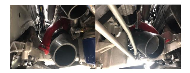
Step 12: At this time we recommend placing the Driver's and Passenger's Side Cold Side tubes (Parts G and H) into their rough positions. The Passenger's side Cold Side tube can be tricky to get into place if not done at this time so we recommend hanging in into position now. Attach the supplied Straight 2" silicone couplers (Parts: V) to the bottom ends of the Cold Side tubes and secure onto the tube using the supplied 2" T-bolt clamps (Parts: W)
