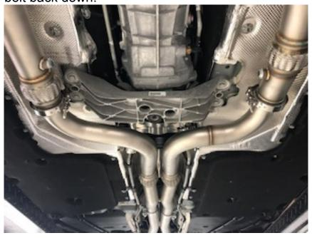
**Step 20:** Slide the (2) Exhaust Sleeve clamps (Parts: BB) over the (2) exhaust tubes exiting your rear mufflers.
