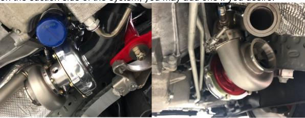
**Step 18:** Installation of the exhaust downpipes. Attach Driver's Side Downpipe (Part C) to the outlet of the installed Driver's Side Turbocharger using the supplied 3" V-band clamp that came with the Turbocharger.
