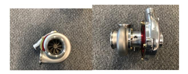
**Step 14:** With the Turbochargers now clocked properly, still leave them loose to test fit in the vehicle. Attach the turbochargers to installed Turbo Exhaust Manifolds (Parts A and B) via the supplied 2.5" V-band Clamps that came with the Turbochargers
