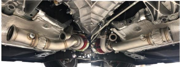
**Step 19:** Install the exhaust Mid-Pipe (Part: E) which is 2-piece bolted together to the ends of the Exhaust Downpipes Parts C and D using (2) of the supplied 3" V-band Clamps (Parts: Z). If you leave the bolt loose that connects the 2 pieces of the Exhaust Mid-pipe together it will make installation easier. Once all aligned properly you can then tighten that bolt back down.
