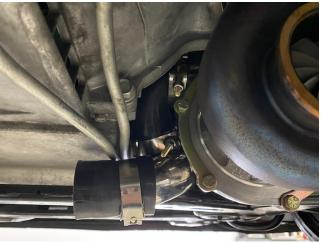
**Step 18:** Install the cold side connection tube **Part**: **H** from the DS compressor outlet into the cold side connection tube assembly using (2)
