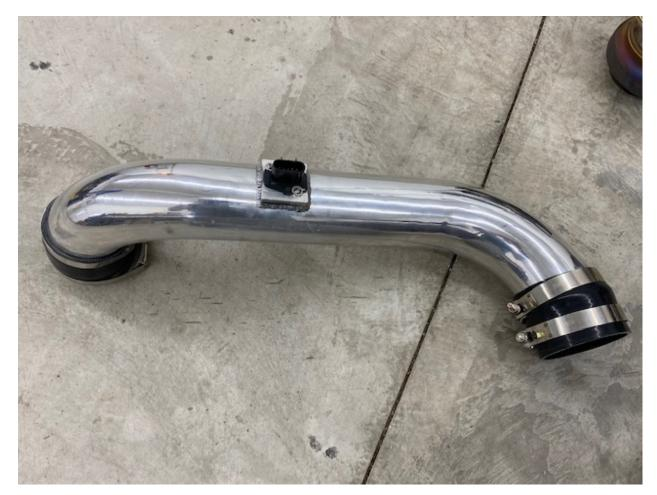
Step 26: Attach MAF loaded cold side tube Part: M to Cold side Tube Part: L via straight 3.5" Coupler. Attach the other end to the throttle body at the previously installed 4" to 3.5" reducing coupler on the throttle body. Attach the other end of Cold side tube Part: L to the intercooler using a straight 3.5" to 3" Reducing coupler. If using the larger HSI-6 intercooler this will use a straight 3.5" coupler.
