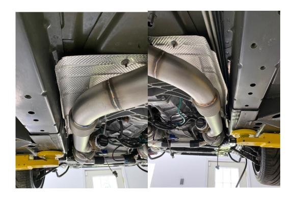
Now you can install the X-pipe, Part: E which mounts to the vehicle using supplied holes and (2) M10x1.5 bolts. Attach the downpipes into the X using the supplied 3" V\_band Clamps. On the back end of the X, the DS Mid-pipe Part: F can be hung in the OEM hanger and attached into the end of the X pipe. Repeat for Part: G on the Passenger side. This will now take your exhaust all the way back to the popular Axle-Back connection.
