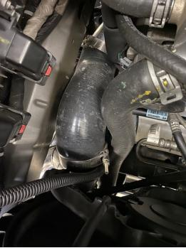
Photo below shows Charge tube Part: K in satin black coating routing into the intercooler.
