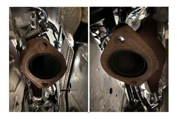
**Step 13:** Install Driver's Side Hot-pipe **Part**: A to your Driver's Side Factory Manifold using the supplied gasket and the Supplied M10x1.5 Studs with the supplied M10x1.5flange nuts. Use some red loc-tite on the threads of the studs into **Part**: A. A bead of copper RTV around the gasket is recommended also as it helps ensure a perfect leak-free seal!
