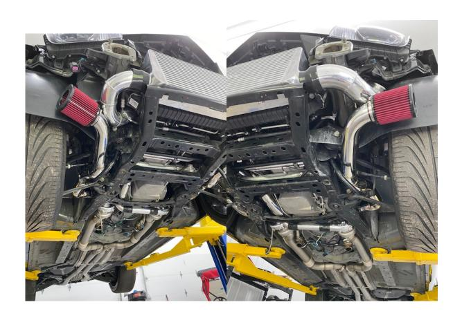
**Step 30:** Back under the car now inspect all of your connections and clearances. Ensure all charge and cold-side tubes are fully inserted into their couplers and the clamps are installed BEHIND the bead-rolls on each tube to prevent blowing off. Ensure nothing is touching any hot-side components or Turbo Assembly as if it is, it will melt! Make sure you have proper clearance in all areas, everything is secure, tight, and most of all SAFE!
