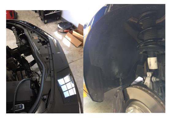
Step 7: Remove the front Bumper bar via the (6) 13mm bolts
