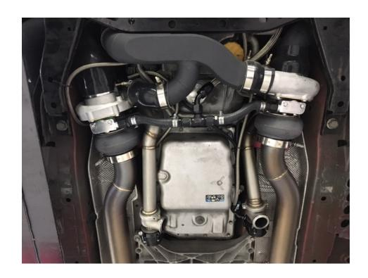
Step 35: (Oil cooled turbos only) Oil Drain Installation. We recommend running a -10an line from the Scavenge pump inlet down to the turbocharger area and into check valve and then a -10an Tee or Y fitting. From the other 2 ports on your Tee or Y fitting run a line to each turbocharger drain. We recommend using our Low profile oil drain flanges as shown above. From the outlet of the scavenge pump we recommend running a -10an hose to the oil fill cap for easy return.
