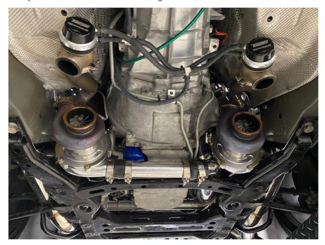
**Step 19:** On the Passenger's Side some massaging of the Transmission Cooler hard-lines is to be expected. See the photos below on a manual transmission vehicle how we gained clearance by simply bending out of the way, this needs to be done on automatic transmission equipped vehicle as well. This is not difficult, just use some care as to not pinch the lines during bending.
