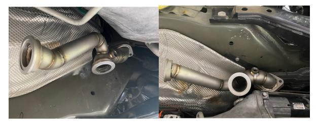
**Step 15:** Loosen the (8) outside bolts on your Turbocharger's Compressor covers as well as the (6) outside bolts on your
