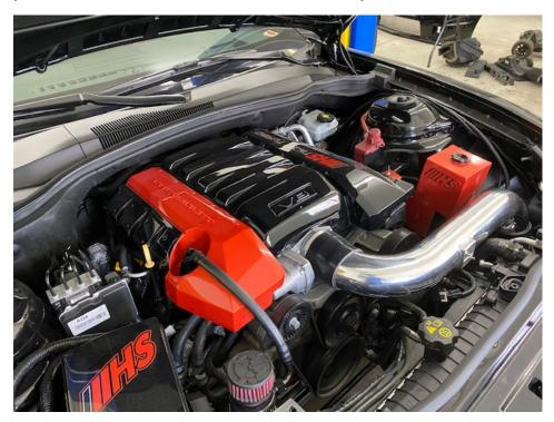
**Step 51:** Ensure your set-up has a proper fuel system to support the new power (If installing new Injectors, do NOT run the car without the computer flashed for the larger injectors). If running the car prior to tuning do NOT get into any boost prior to tuning or you WILL damage the engine. Proper fueling and a professional dyno tune is REQUIRED to safely run this system on your vehicle, remember.
