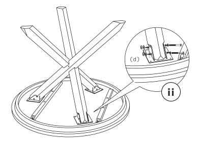
3. Tighten the legs as in picture above with bolt nut and ring as in detail (ii)
