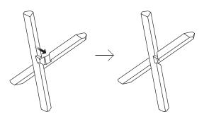
1. Instal the legs as in picture above and tighten with bolt and rings as in detail (i)  $% \left( {\left( {{{{\bf{n}}_{\rm{s}}}} \right)_{\rm{s}}} \right)$
