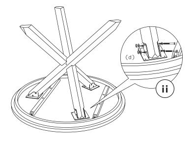
Tighten the legs as in picture above with bolt nut and ring as in detail (ii)
