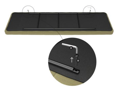
Attach the long leg (B) to the seat frame (A). Insert two metal bolts (D) and use the Allen Key (E) for tightening. Avoid fully tightening all the metal bolts until all components are properly aligned in place, making sure that the metal legs are in the correct alignment.
