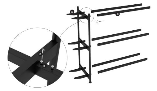
While one holds the other frame upright, the other carefully slides the bars into place and mounts them with the socket head screws.
