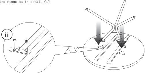
2. Instal the legs into the table top and tighten with nut and ring as in detail (ii)
