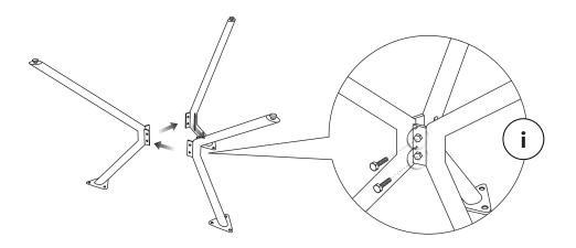
1. Instal the legs as in picture above and tighten with bolt and rings as in detail (i)
