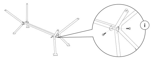
1. Instal the legs and leg connector as in picture above and tighten with bolt as in detail (i)
