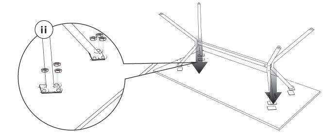
2. Instal the legs into the table top and tighten with nut as in detail (ii)
