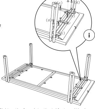
2. Tighten the legs into the table top with rings and bolts as in detail (i)
